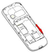
4) With the metallic part of the battery facing the metallic part in the battery slot, press the battery down until it locks into place, then fix its back cover
