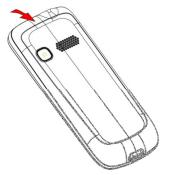
2) Insert the SIM card into the SIM card slot lightly with the corner cutting of the card aligning to the notch of the slot and the gold plate of the card facing downward, till the SIM card cannot be pushed in further.
