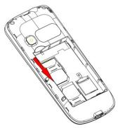
3) To install the T-Flash card, open its latch, place its indented side downward, insert the card into the card slot, and then close the latch.
