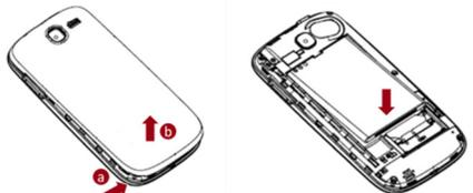
**Caution:** Install according to the illustration above to avoid breaking the battery connectors.
