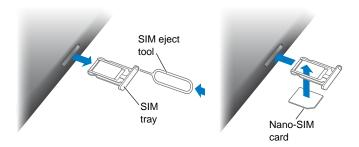
Open the SIM tray. Insert the SIM eject tool into the hole on the SIM tray, then press firmly and push the tool straight in until the tray pops out. Pull out the SIM tray to install or replace the SIM card. If you don't have a SIM eject tool, try the end of a small paper clip.
