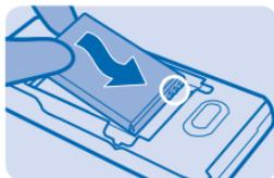
5. Press the back cover down until it locks into place. To switch the phone on, press and hold the power key
