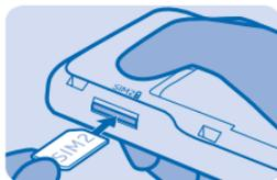
3. To remove the SIM, push the card in until it's released, then pull it out.
