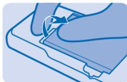
3. Lift the cover of the SIM1 holder, and put the SIM in, contact area face down.
