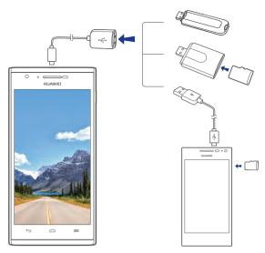
To connect your phone to another phone, make sure that the phone you wish to connect to supports the USB mass storage function and has a microSD card installed. To establish the connection and read data stored on the microSD card:
