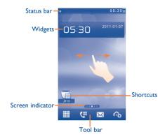
The Home screen is provided in an extended format to provide you with more space for adding widgets and shortcuts. Slide the Home screen horizontally left and right to get a complete view of the Home screen. Small dots at the bottom of the screen indicate which screen you are viewing.
