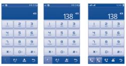
Enter the desired number on the on-screen keypad directly or select a contact from Call log or Contacts by touching or or respectively, then touch to place the call. Press to return to the Home screen. If you want to return to the call screen, touch to return to the call screen.
