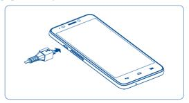
Connect the battery charger to your phone and mains socket respectively, LED indicator will light while charging.
