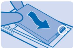
5. Press the back cover down until it locks into place. To switch the phone on, press and hold the power key
