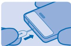
2. Slide the memory card into place with the contact area face down.
