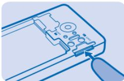
If you only have one SIM card, put the card into the SIM1 card holder. Some features and services may only be available when using the SIM card in the SIM1 card holder. If there is a SIM card only in the SIM2 card holder, you can only make emergency calls.
