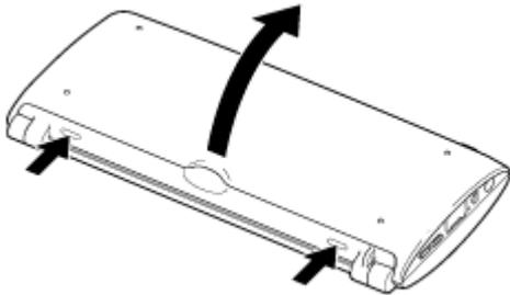
2. Orient the contacts as shown, and then insert the battery pack.
