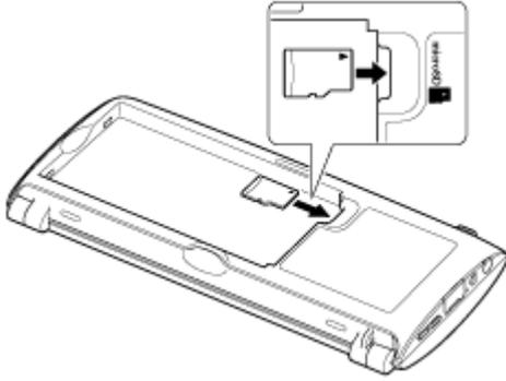
4. Carefully slide the microSD memory card into the slot until it clicks into place.
