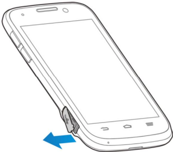
2. Connect the adapter to the charger/micro-USB jack. Ensure that the adapter is inserted with the correct orientation. Do not force the connector into the charging jack.
