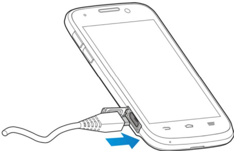
3. Connect the charger to a standard AC wall outlet. If the phone is on, you'll see a charging icon, such as
