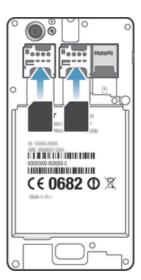
Remove the battery cover, then insert the SIM card into its slot with the goldcoloured contacts facing down.
