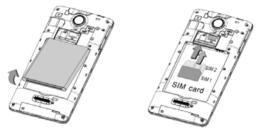
3. Insert the battery and place back the rear cover.
