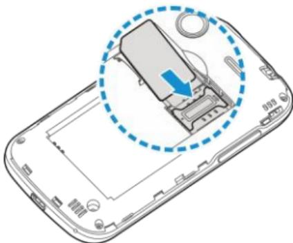
3. Open the microSD card holder, hold your microSD card with the metal contacts facing down and slide it in, and then close the card holder.
