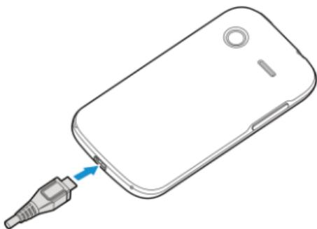
2. Connect the charger to a standard AC wall outlet. If the phone is on, you'll see a charging icon (
