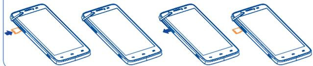
Insert the microSD card with golden contact facing downwards into the slot. To remove the microSD card, gently press and slide it out.
