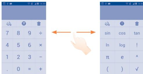
Enter a number and the arithmetic operation to be performed, enter the second number, then touch “=” to display the result. Touch  $\frac{1}{2}$  to delete digits one by one, touch and hold  $\frac{1}{2}$  to delete all at one time.
