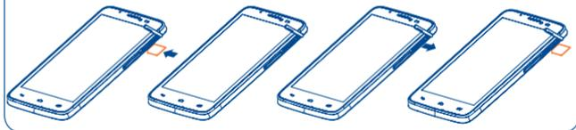
To install, place the SIM card chip facing downwards, and then slide it into its slot. Make sure that it is correctly inserted. To remove the card, press and slide it out.
