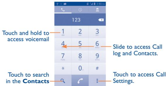
Enter the desired number from the keyboard directly or select a contact from Contacts or Call log by sliding or touching tabs, then touch to place the call.
