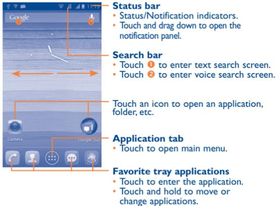
Home screen is provided in an extended format to allow more space for adding applications, widgets, etc. Slide the Home screen horizontally left and right to get a complete view of Home screens.
