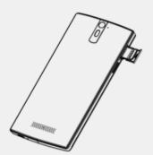
Step 3: Place your SIM card into the tray with the metal surface facing up
