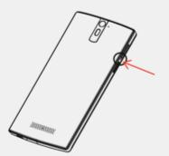
Step 1: Use the special pin and insert it into the hole next to the SIM tray to push it out
