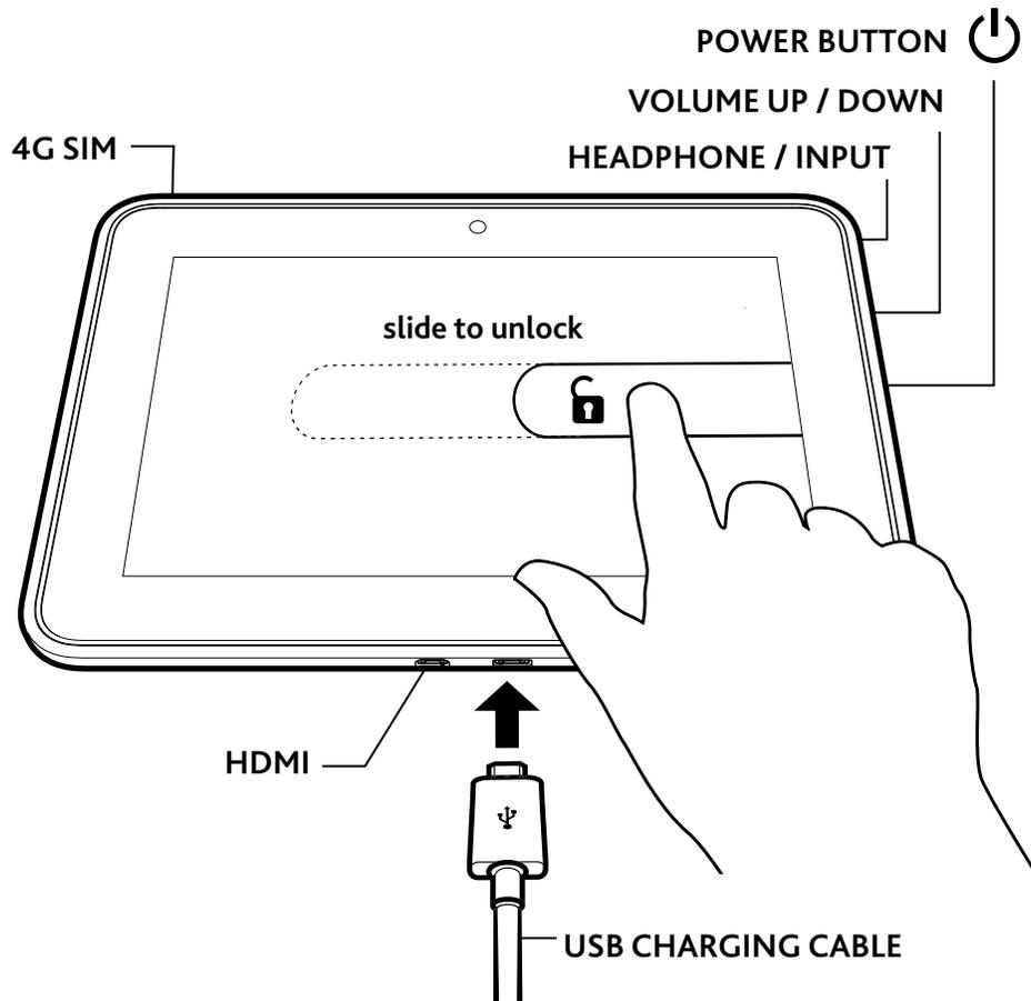
To charge your Kindle, connect it to the USB charging cable as shown. Connect the opposite end of the USB charging cable to a Kindle Power-Fast accelerated charging accessory (sold separately), or other USB power adapter. To learn more about charging accessories, visit [www.kindle.com/support/charging](http://www.kindle.com/support/charging).
