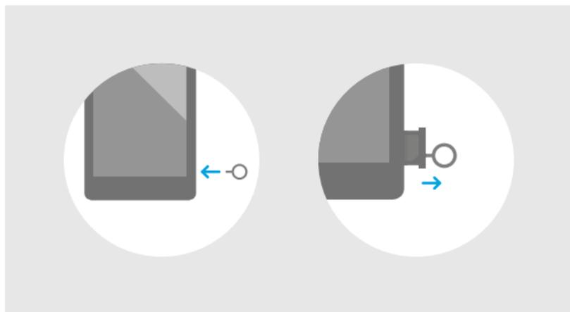
4. Remove the tray and place the micro SIM card inside it, with the angled corner fitting snugly into the angled corner of the tray.
