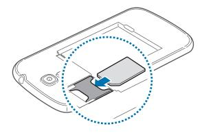
3 Push the SIM or USIM card into the slot until it locks in place.
