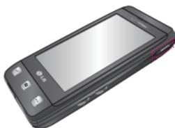
2. Push the microSD card into the slot with its gold contacts facing down until it clicks into place and then replace the slot cover.
