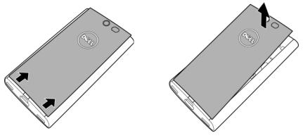
**NOTE:** Do not turn on the phone when the back cover is removed.
