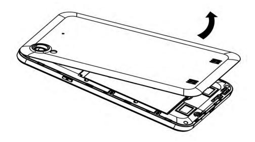
2, Take off the battery, put the SIM card into the corresponding card slot
