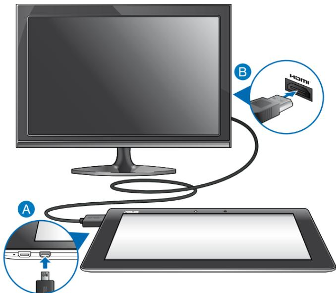
To connect an HDMI-compliant display:
