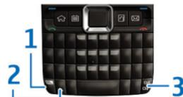
1 — Function key. To insert digits or characters printed at the top of keys, press and hold the function key and press the corresponding key, or press and hold the corresponding key only. To enter only the characters printed at the top of keys, press the function key twice quickly.
