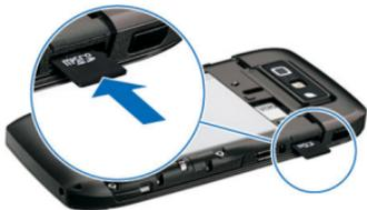
2. Insert the memory card in the slot with the contact area first. Make sure that the contact area is facing the connectors on the device.
