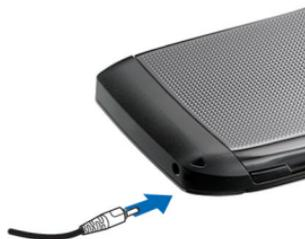
3. When the battery is fully charged, disconnect the charger from the device, then from the wall outlet.
