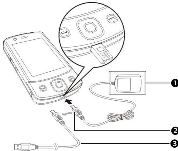
1. It will take about 8 hours to fully charge the battery after the first time you open the package. Subsequent charging will only take about 3 hours. After charging, you can disconnect the AC adapter and carry the Pocket PC around portably. To maintain smooth operation, charge the power regularly.
