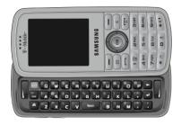
When you slide the phone open, the display rotates from a vertical viewing mode to a horizontal viewing mode.
