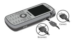
Note: The previous illustration displays the incorrect method for connecting the charger. If attempted, damage to the accessory port occurs therefore voiding the phone's warranty.
