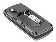
Note: If the card is not inserted correctly, the phone does not detect the SIM card. Remove the battery and re-orient the card back into the slot.
