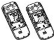
Press the release spring (1), and slide out the SIM card (2).
