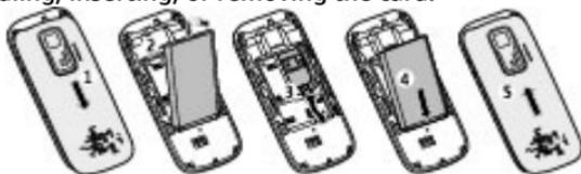
1. Press and slide the back cover towards the bottom of the phone, and remove it (1).
