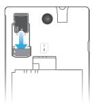
Remove the battery cover and insert the memory card with the gold-coloured contacts facing down.
