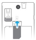
Remove the battery cover, then insert the SIM card into its slot with the goldcoloured contacts facing down.
