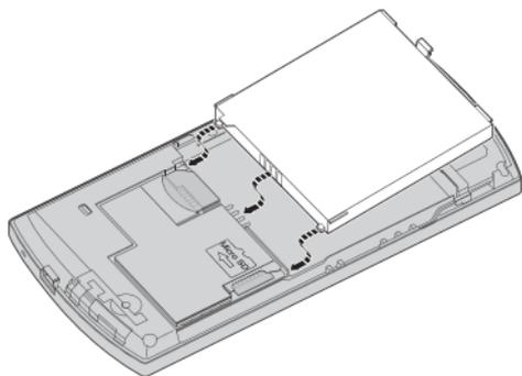
Insert the tabs on the bottom of the battery cover into the slots in the smartphone.
