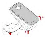
In the lower left corner of the phone, use your finger to open a gap between the back cover and the phone carefully. In the direction shown by the arrow indicator (b), use your hand to remove the entire back cover.
