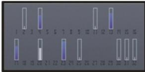
If your device has found satellites, a bar for each satellite is shown in the satellite info view. The longer the bar, the stronger the satellite signal. When your device has received enough data from the satellite signal to calculate your location, the bar colour changes.
