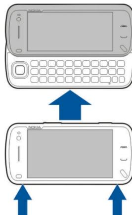
Your device has a full keyboard. To open the keyboard, push the touch screen up. In all applications, the screen rotates
