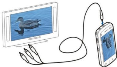
All audio, including active calls, stereo video clip audio, keypad tones, and ringing tone is routed to the TV when the Nokia Video Connectivity Cable is connected to the device. You can use the device microphone normally.
