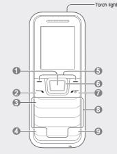
Confirm key Select the highlighted menu option or confirm an input; In Idle mode, access Menu mode Depending on your service provider or region, the key may perform differently
