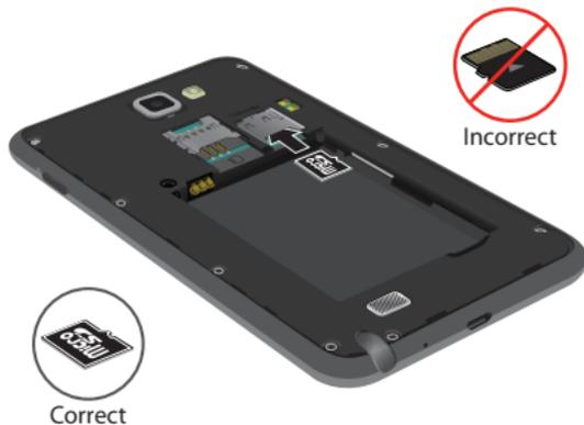
2. To remove, push on the memory card until it clicks and is released. Then grasp the memory card and remove it from the phone.
