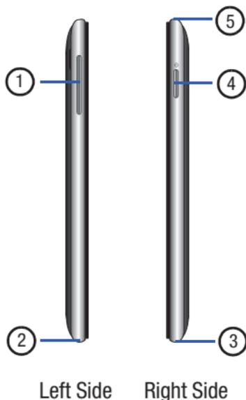
1. **Volume keys:** allow you to adjust the ringer volume while in standby mode or adjust the voice volume during a call. When receiving an incoming call, briefly press down either volume key (
