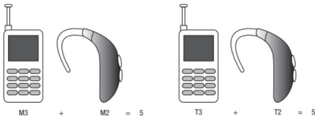
If a hearing aid meets the M2 level rating and the wireless mobile device meets the M3 level rating, the sum of the two values equal M5. This is synonymous for T ratings. This should provide the hearing aid user with “normal usage” while using their hearing aid with the particular wireless mobile device.
