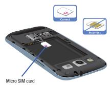
Make sure that the card's gold contacts face into the phone and that the upper-left angled corner of the card is positioned as shown.
