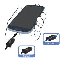
Note: This illustration displays both the correct and incorrect orientation for connecting the charger. If the charger is incorrectly connected, damage to the accessory port will occur therefore voiding the phone's warranty.
