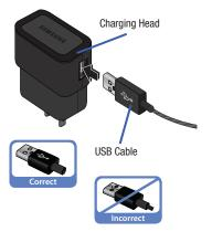
Note: Verify that the battery is installed prior to connecting the wall charger. If both the wall charger is connected and the battery is not installed, the handset will power cycle continuously and prevent proper operation. Failure to unplug the wall charger before you remove the battery, can cause the device to become damaged.
