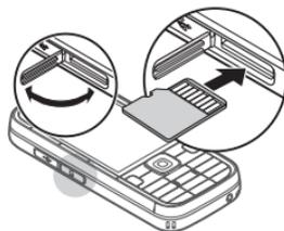
2. Insert the memory card in the slot with the contact area first. Ensure the contact area is facing the connectors on the device.
