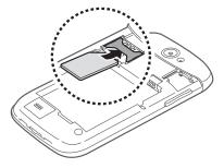
The antenna is located below the memory card slot. Do not remove the protective tape covering the antenna, as this can damage the antenna.
