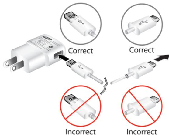
2. Insert the USB cable into the device's Charger/Accessory Port (2).
