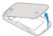
Insert the battery by aligning the gold contacts on the battery with the gold contacts in the battery compartment. Gently push down on the battery until it clicks into place.
