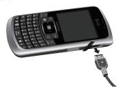
Warning!: You must unplug the adapter before removing the battery from the phone during charging to avoid damage.
