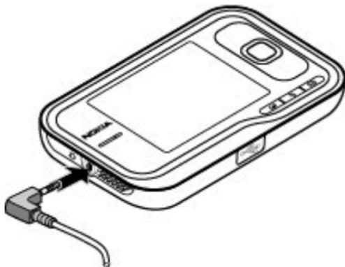
Do not connect products that create an output signal as this may cause damage to the device. Do not connect any voltage source to the Nokia AV Connector.
