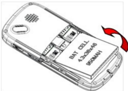
■ When inserting the battery, insert the metal teeth at the top of
