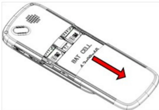
■ Lift the battery from the bottom and take the battery out.
