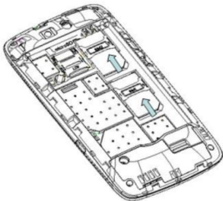
3. Finally insert the battery and replace the rear cover of the mobile phone.
