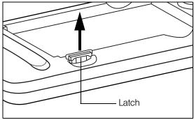
4. Gently pull the microSD card out from the slot, and then press the latch back to lock position.
