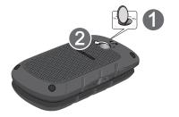
Use the groove at the top left corner of the cover (3) to lift the cover up and away from the back of the phone (4).
