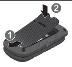
**Note:** The battery must be properly installed before charging the battery or switching on the phone.
