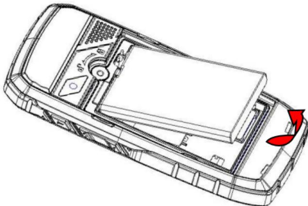
■ When installing the battery, insert the metal teeth at the top of the battery into corresponding slot of the mobile phone, and then press the battery down to install the battery in place. The battery must be ensured to be installed before power on.
