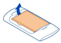
4 Lift the SIM card holder cover, make sure the contact area of the SIM card is facing down, and place the card in the holder.
