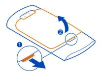
3 Remove the battery, if inserted.
