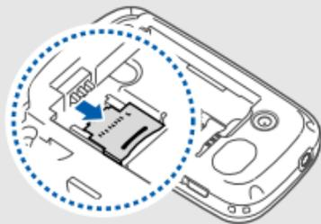
3. Lift the memory card holder and insert a memory card as shown.
