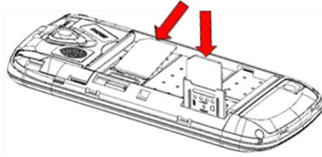
**Note:** The SIM-card slot is at the downside of the battery.
