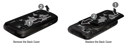
To replace the cover, slide the cover forward (1), then press down gently until it snaps into place (2).
