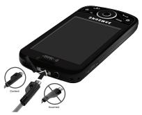
Note: This illustration displays both the correct and incorrect orientation for connecting the charger. If the charger is incorrectly connected, damage to the accessory port will occur therefore voiding the phone's warranty.
