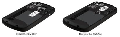
2. To remove the SIM Card, carefully slide the SIM card out of the SIM card socket.
