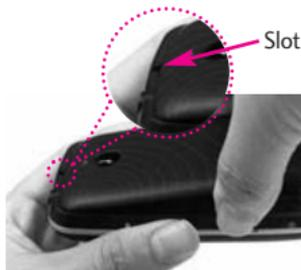
1. Align the battery cover slightly lower than the top edge of the phone. Make sure that the hooks on the battery cover are placed in the phone's slots.
