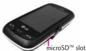
1. Locate the microSD slot on the right side of the phone, then uncover the slot.
