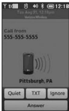
1. When the phone rings and/or vibrates, unlock the touch screen by dragging **UNLOCK** to the right then touch **Answer**, or press the **Send Key**
