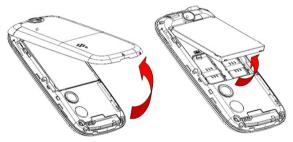
When inserting the battery, insert the metal teeth at the top of the battery into corresponding slot of the mobile phone, and then press the battery down to insert the battery in place. The battery must be correctly inserted before powering on.
